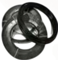
3/8" POLYAMIDE PIPE (NYLON) COLOR: BLACK MAXIMUM PRESSURE: 180BAR BURST PRESSURE: 300BAR
