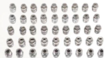
HIGH PRESSURE NOZZLES MATERIAL: SS304 INCH SIZE: 1/4", SPRAY PATTERN: FLAT FAN SPRAY ANGLE: 0 - 65 DEGREES THREAD: BSPT MALE
